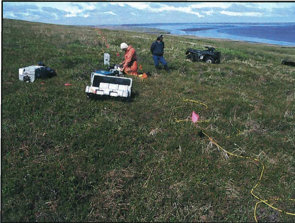
PHOTO 7: ERI EQUIPMENT SETUP ON LINE 1 OF SURVEY
