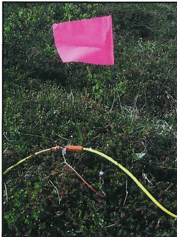
PHOTO 8: ERI MEASUREMENT STATION WITH CABLE AND WIRE LEADING TO STEEL STAKE IN GROUND FOR ELECTRICAL CONDUCTANCE
